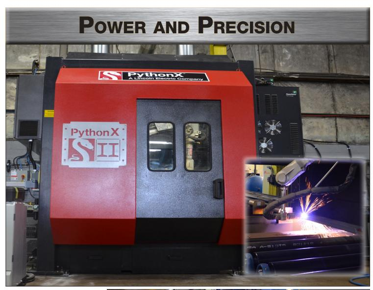
Our latest acquired machine, the PythonX II, is a robotic CNC high definition plasma cutting system. This machine can also perform beam drilling, coping, and piece marking with the capability of fabricating 20,000 lbs. of steel per day. Lincoln Contracting is an AISC certified fabricator, assuring you a quality product with on-time delivery.
