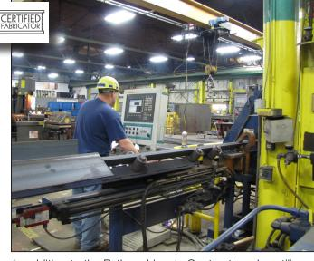
In addition to the Python, Lincoln Contracting also utilizes an Ocean Clipper, a CNC Angle Line, that can process clip angles and long bracing angles. The Clipper completely eliminates manual layout and manual drilling and punching. It produces perfectly accurate clip angles in the fastest possible time, eliminating huge amounts of expensive man hours and errors.
