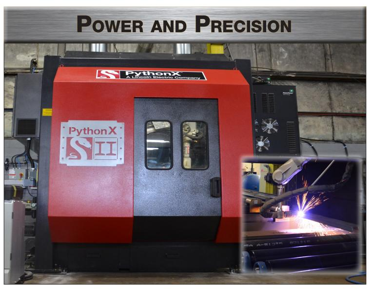
The PythonX II, is a robotic CNC high definition plasma cutting system that has revolutionized structural steel fabrication. More than a machine, the PythonX is the new standard in our modern fabrication shop. This machine can perform beam drilling, coping, and piece marking. LCE has the capability of fabricating 1,000 tons of steel per month as an AISC certified fabricator, assuring you a quality product with on-time delivery.
