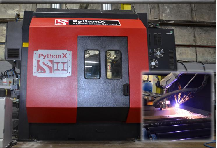
The PythonX II, is a robotic CNC high definition plasma cutting system that has revolutionized structural steel fabrication. More than a machine, the PythonX is the new standard in our modern fabrication shop. This machine can perform beam drilling, coping, and piece marking. LCE has the capability of fabricating 1,000 tons of steel per month as an AISC certified fabricator, assuring you a quality product with on-time delivery.
